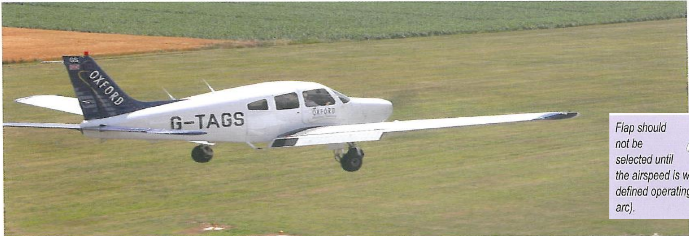
Figure 10.20 Deployment of landing flap.
