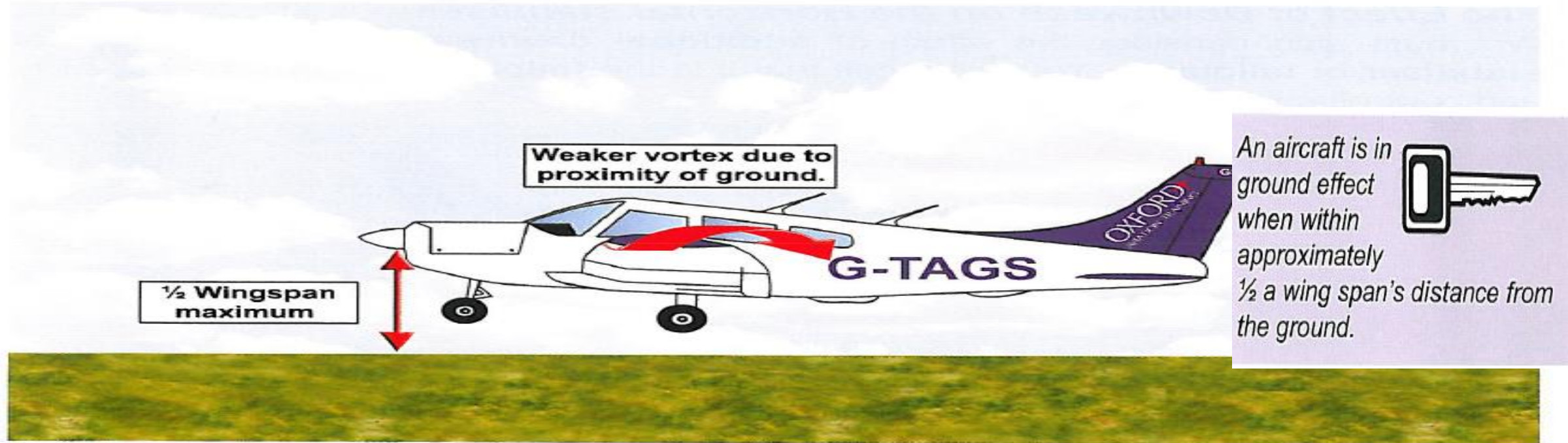
Figure 5.32 Ground effect prevents full development of the wing tip vortices.
