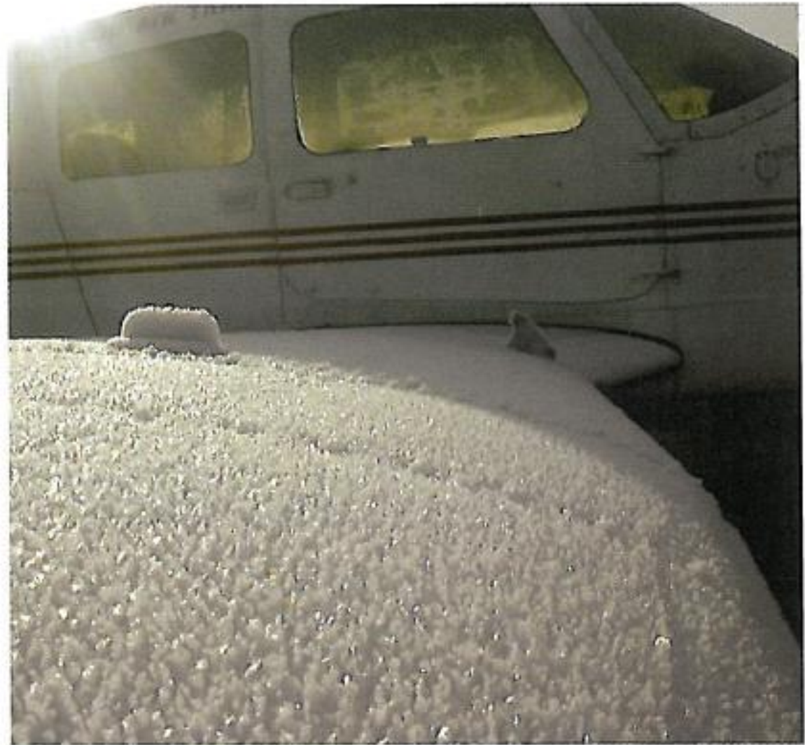
Figure 13.18 Frost, snow and ice on the wings increase stall speed.
