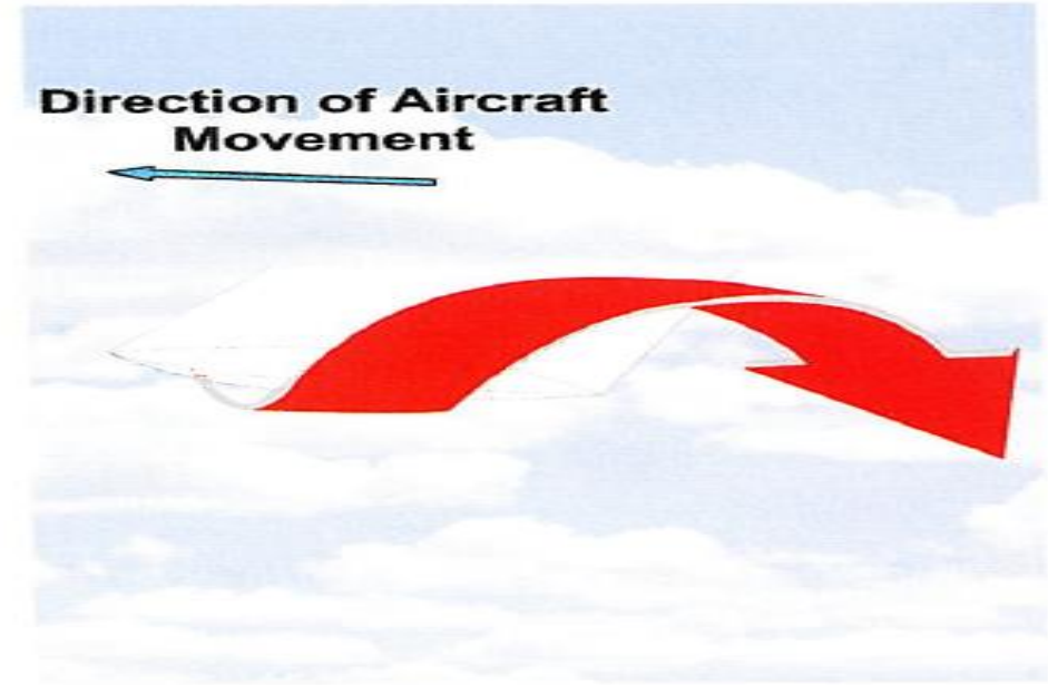
Figure 5.17 The wingtip vortex is particularly large and strong.
