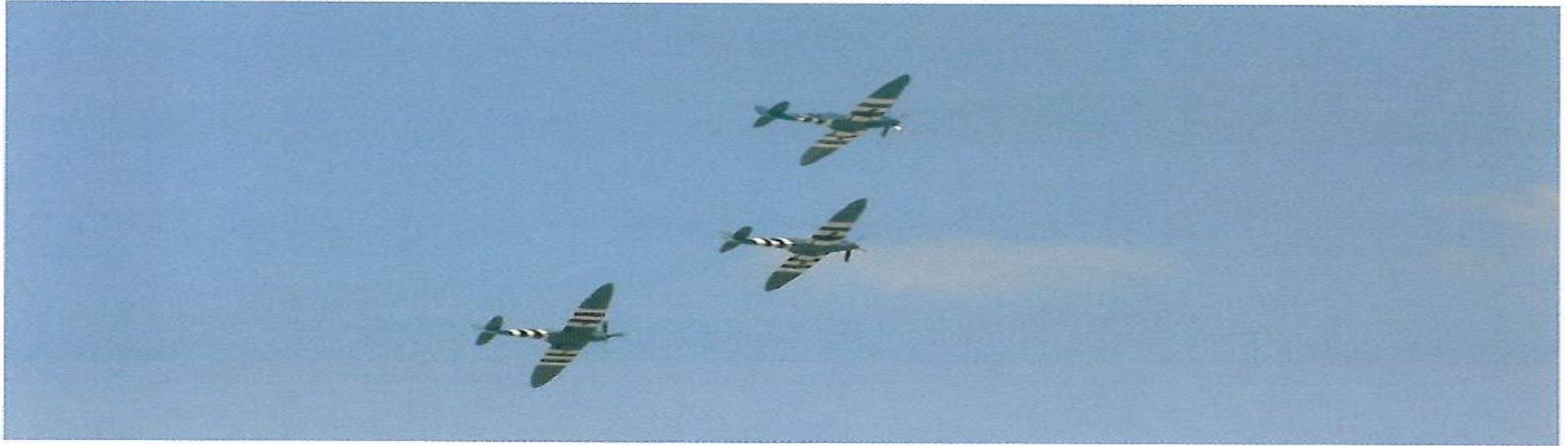
Figure 5.23 Spitfires showing elliptical wing plan form.
