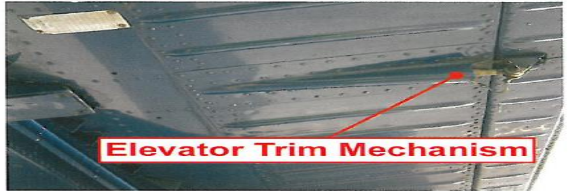
Figure 1.19 Elevator Trim Mechanism.
