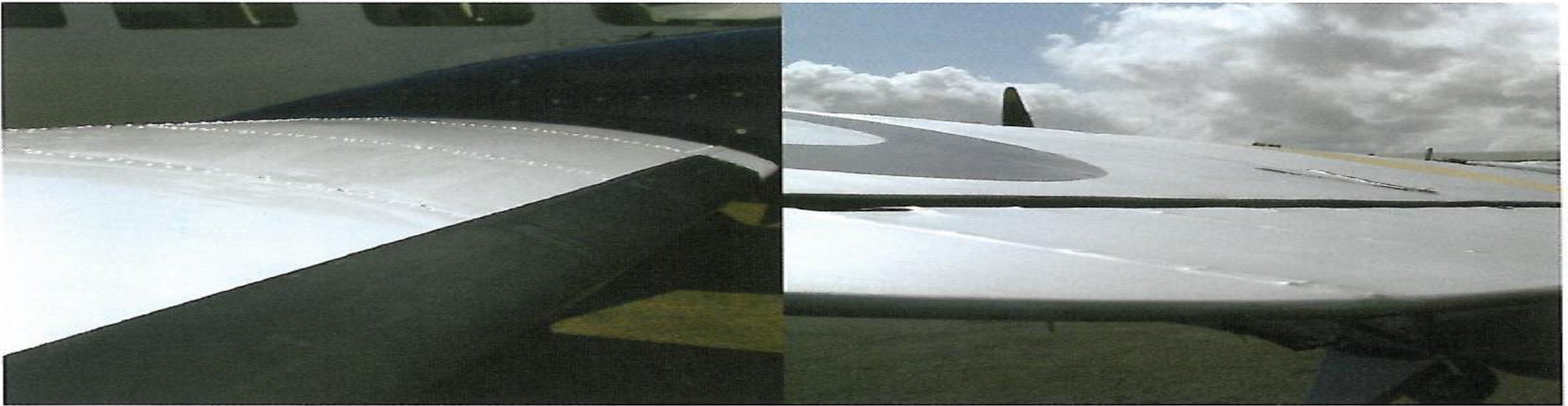
Figure 5.3 The surface area and the surface finish affect skin friction drag.
