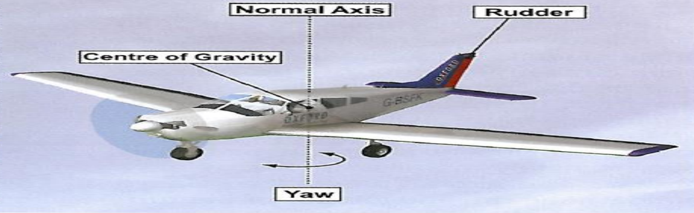
Figure 12.4 The rudder controls the aircraft in yaw, about its normal axis.
