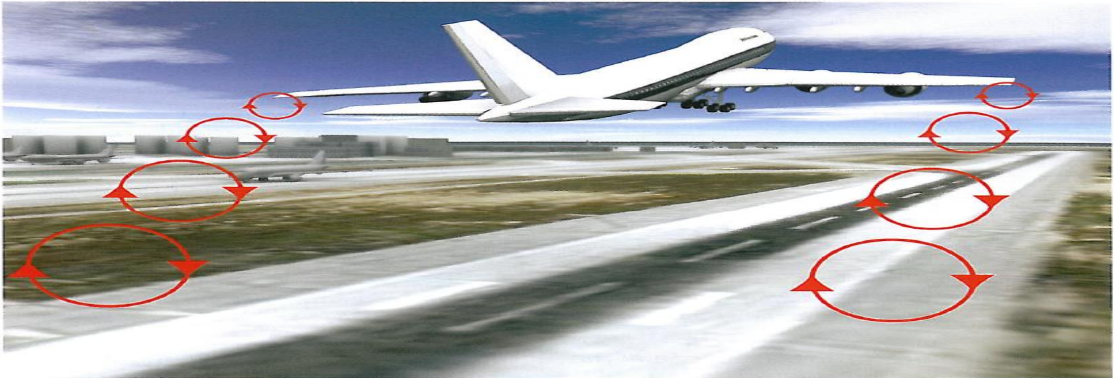
Figure 5.12 The regions of differing pressure, above and below the wings, induce vortices which vary in drag effect with varying angle of attack.
