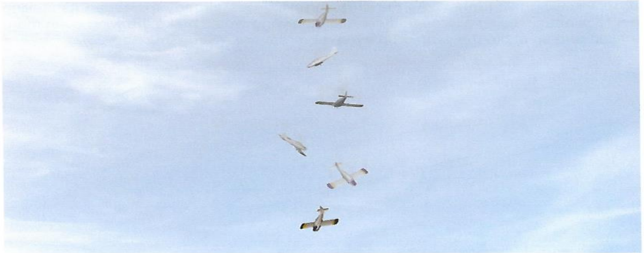
Figure 13.27 The spin is a state of stalled flight with the aircraft in a steep descent, yawing, rolling and pitching at the same time.
