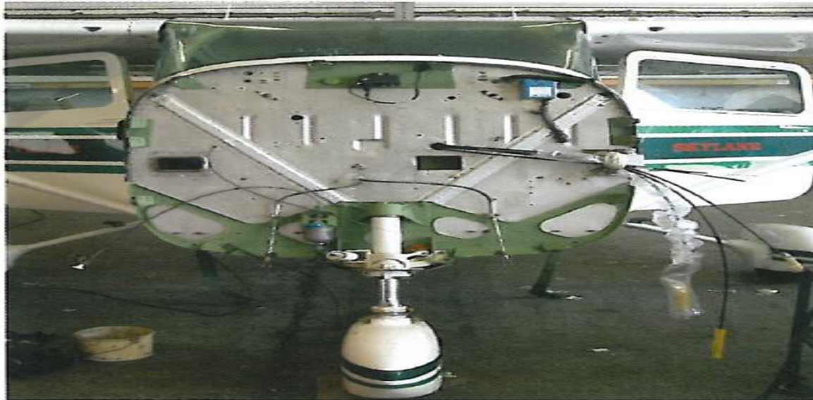
Figure 1.5. An Engine Bulkhead.
