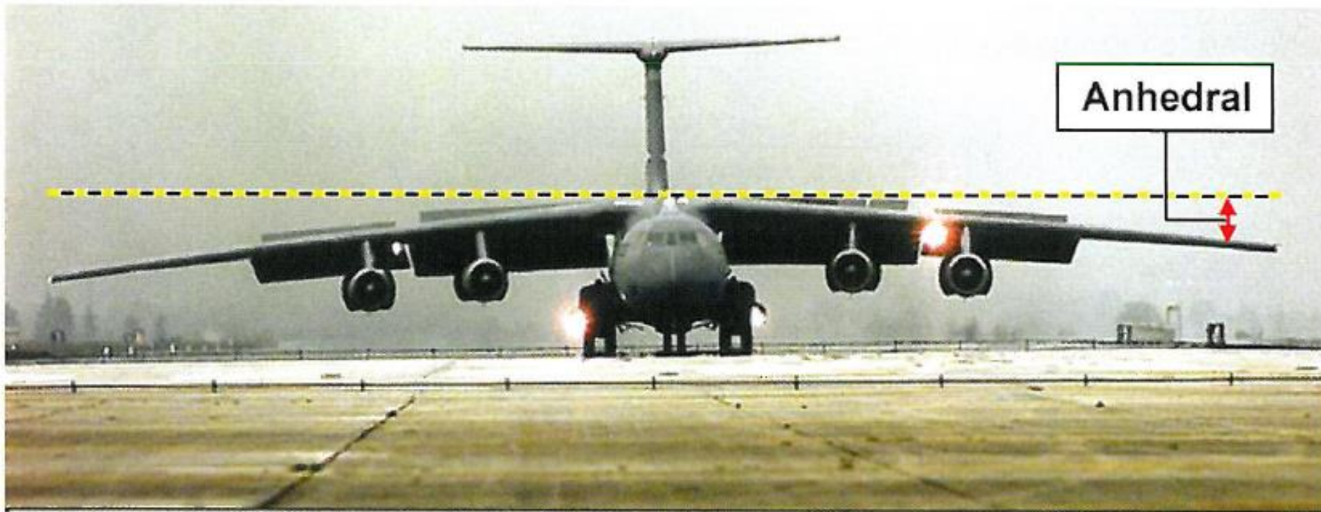
Figure 11.27 Anhedral reduces lateral stability.
