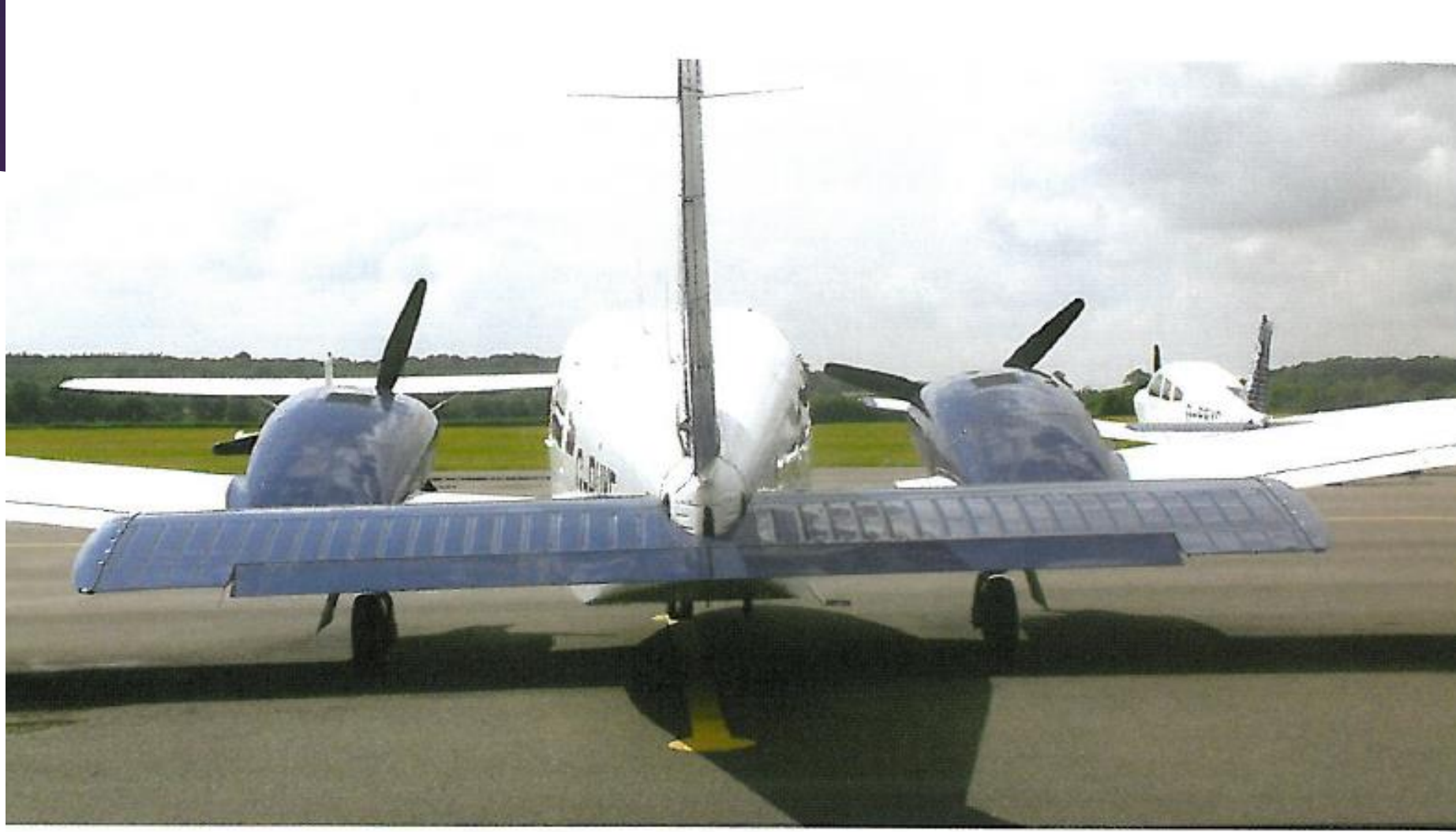
Figure 12.30 Anti-balance tabs are most commonly found on aircraft with all-flying tailplanes or stabilators .
