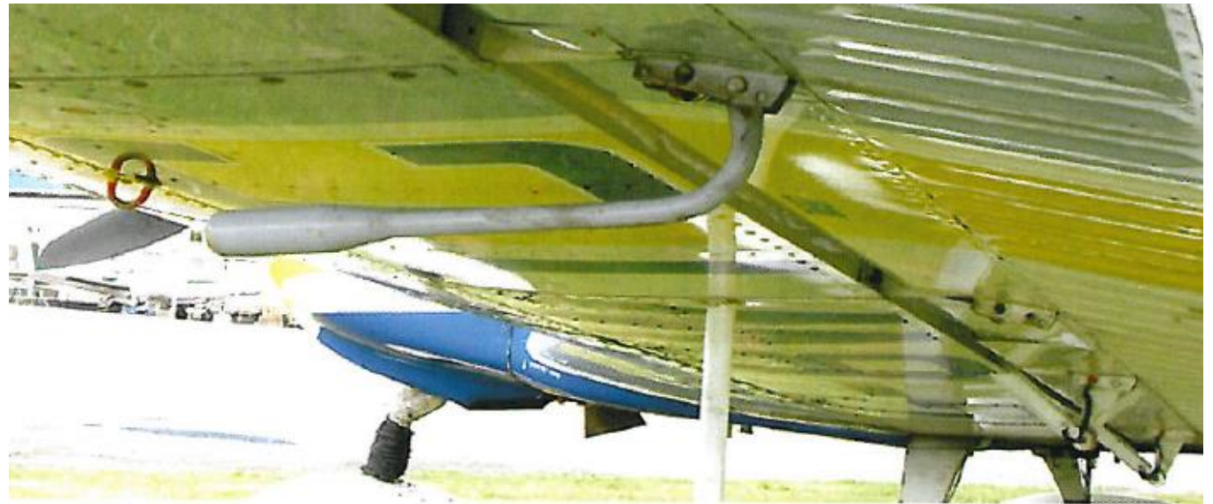
Figure 12.34 The mass balance fitted to the ailerons of a Zlin.
