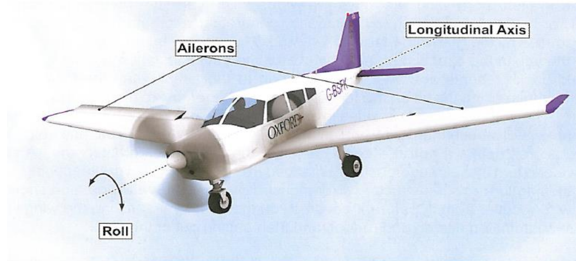
Figure 12.8 Control in roll is achieved with the ailerons.
