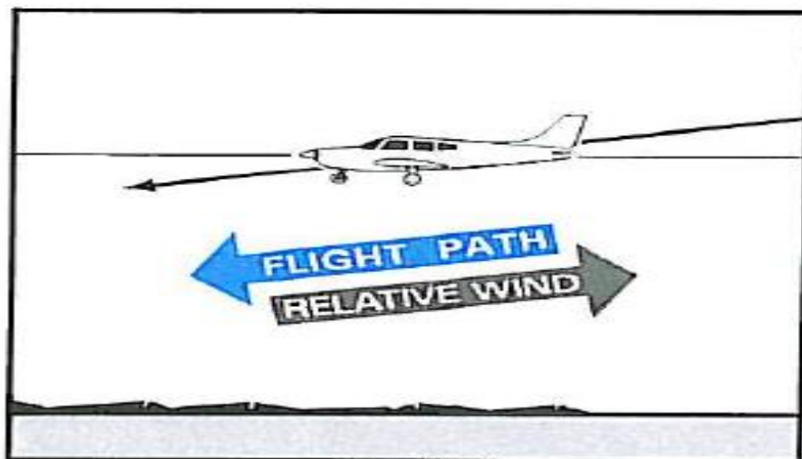
Figure 1-17. This airplane is in a level flight attitude, while the actual flight path is forward and down. Notice that the relative wind is upward and back, parallel to and opposite the flight path.
