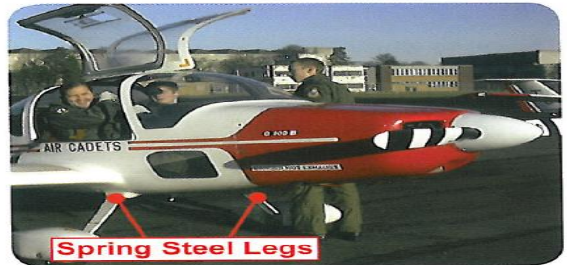
Figure 2.3 Spring Steel Legs.
