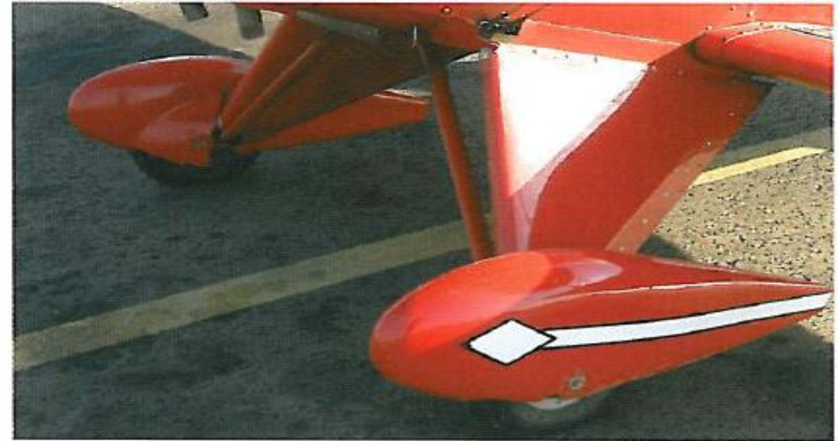
Figure 2.6 Spats, fitted to a Pitts S2a.
