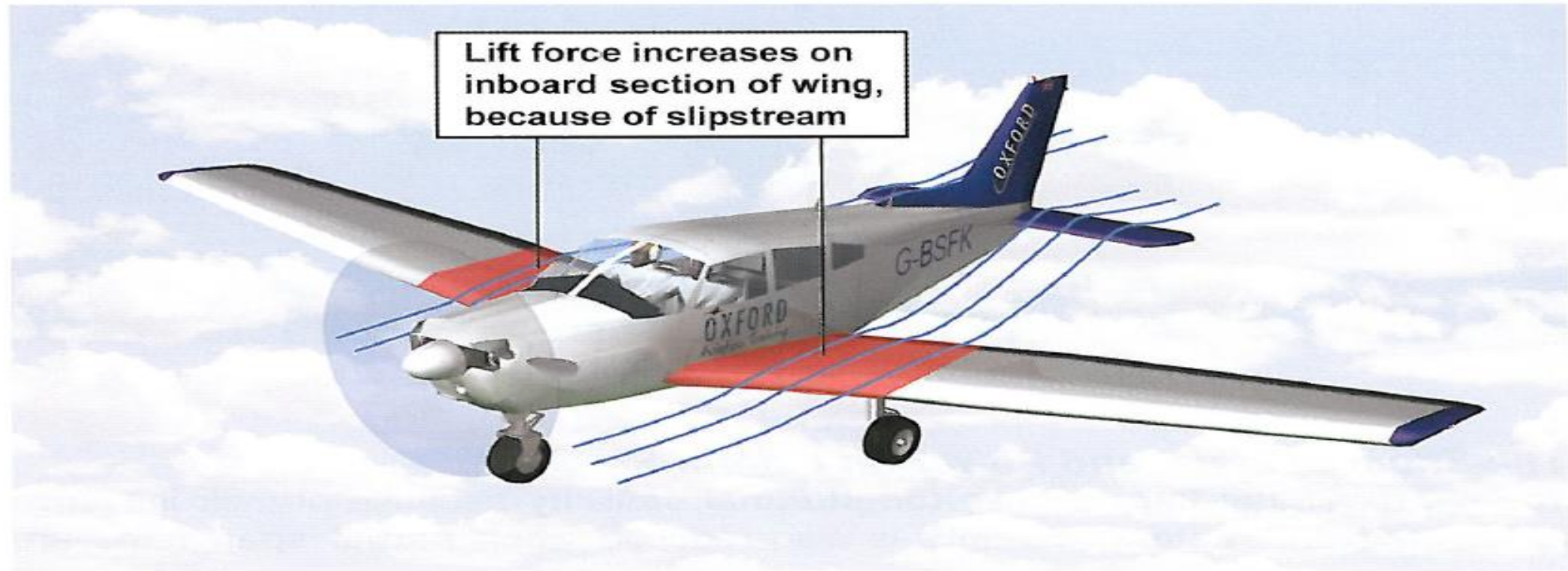
Figure 11.29 High power settings at low forward speed reduce lateral stability.
