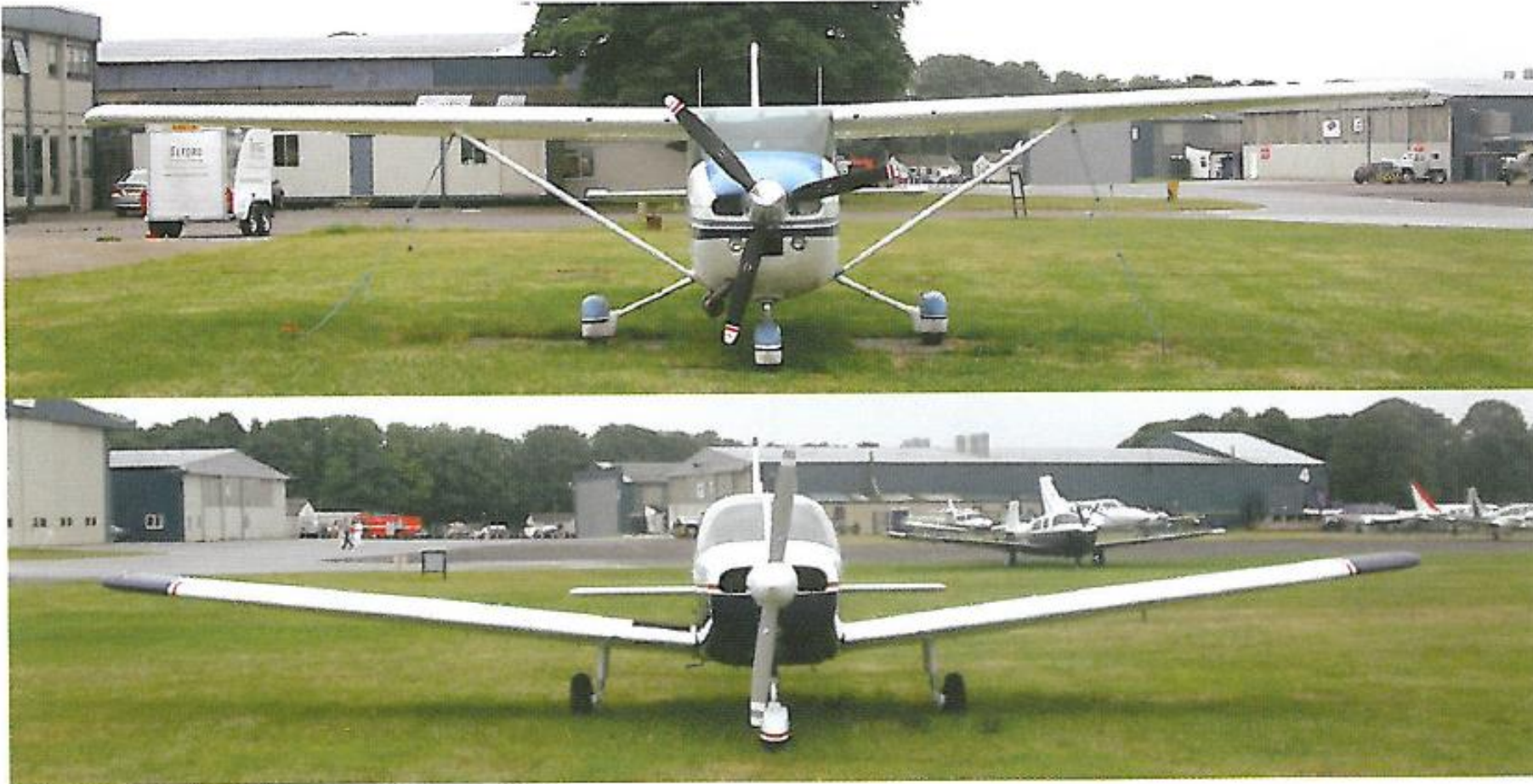
Figure 11.23 The difference in dihedral between low and high wing aircraft.
