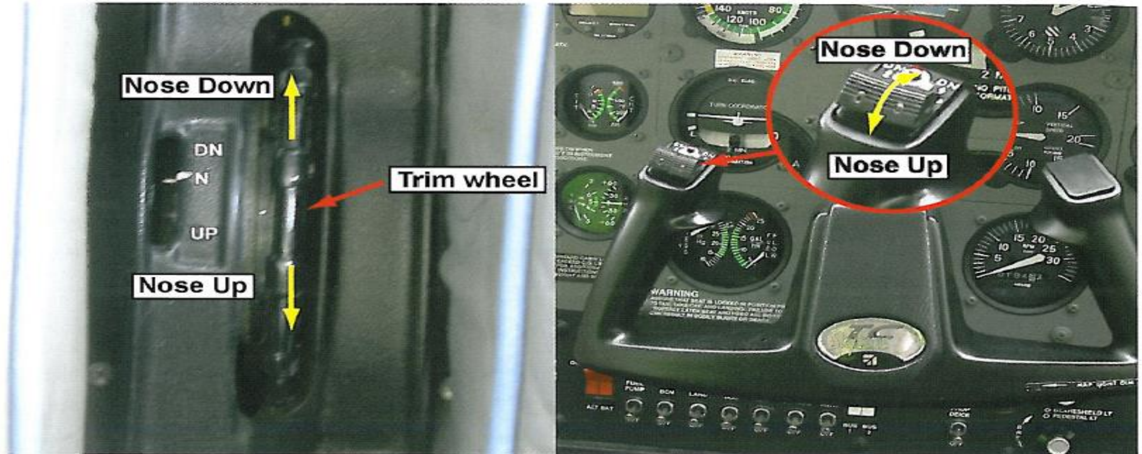
Figure 12.38 Two methods of pilot trim control.
