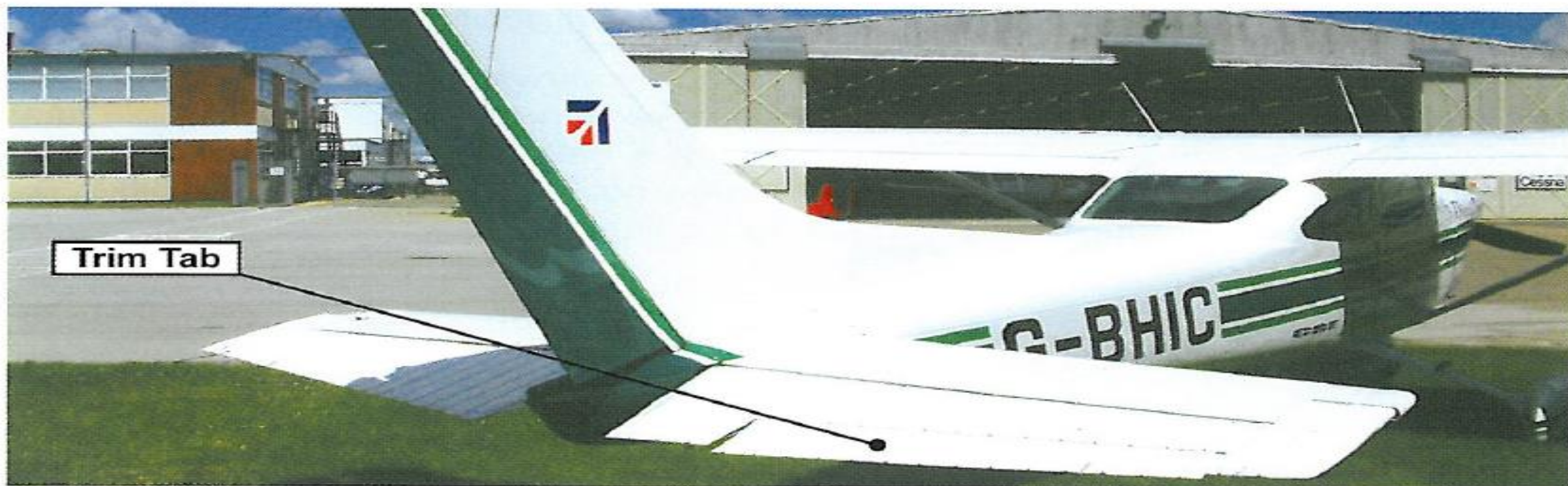
Figure 12.36 An adjustable trim tab fitted to the elevator of a Cessna.
