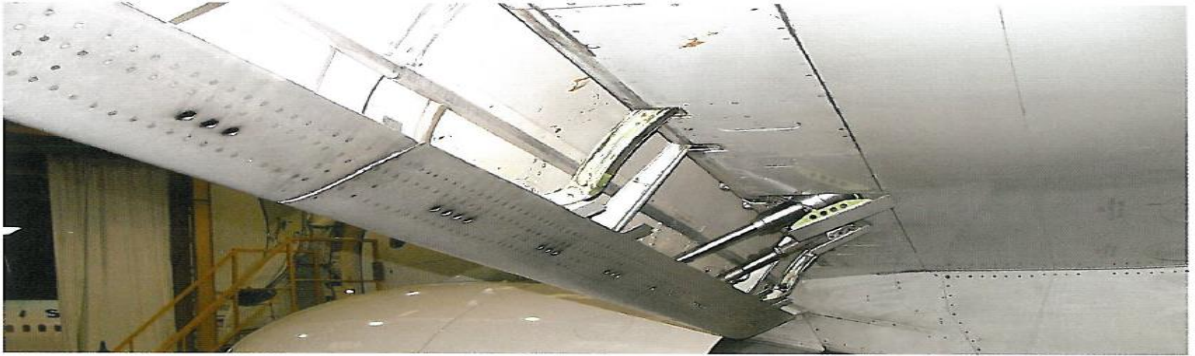
Figure 10.23 A typical leading edge flap on a jet transport aircraft.
