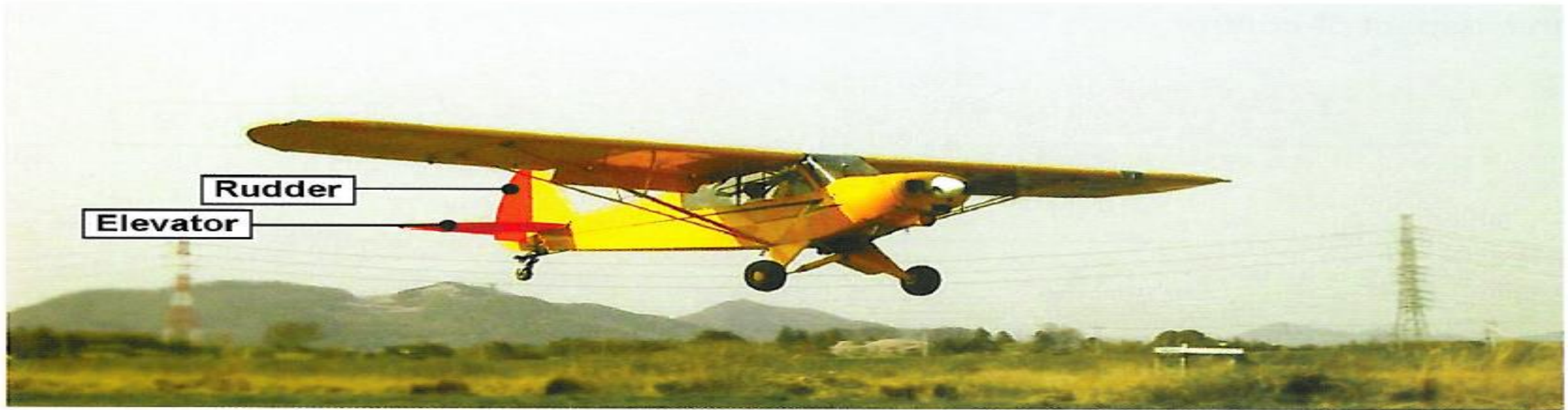
Figure 12.19 Only the rudder and elevator benefit from the propeller slipstream effect. Great care, should, therefore, be exercised by the pilot to retain control over the aircraft in roll, when landing in gusty or cross-wind conditions.
