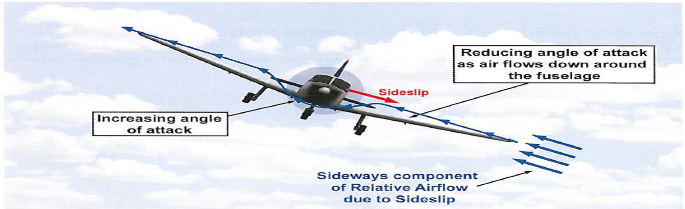
Figure 11.20 Low wing aircraft possess characteristics which reduce lateral stability.
