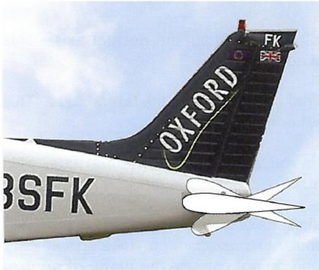
Figure 12.3 A stabilator or all-moving (flying) tailplane.
