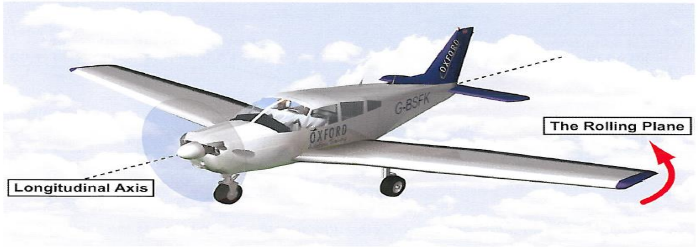
Figure 11.15 Lateral Stability is stability in roll about the longitudinal axis.
