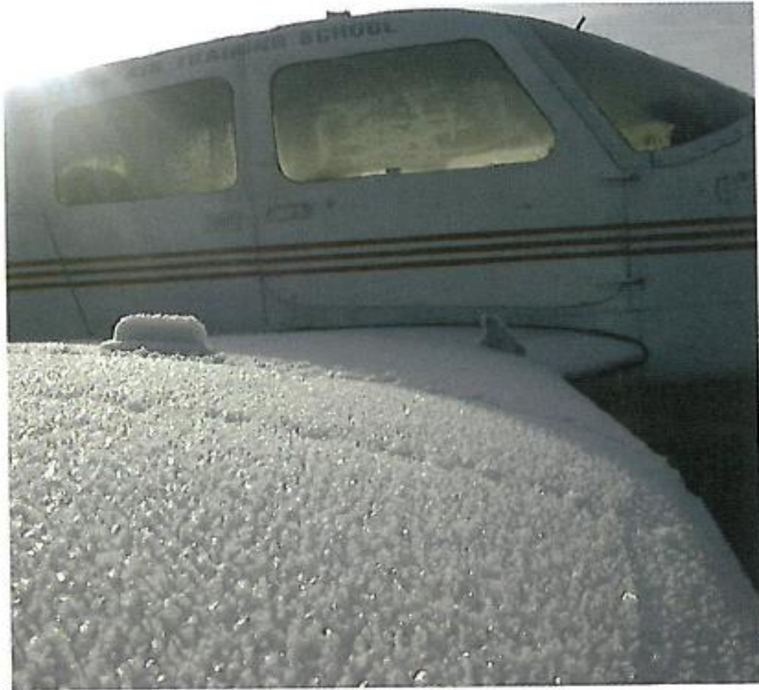
Figure 5.5 The surface area and the surface finish affect skin friction drag.
